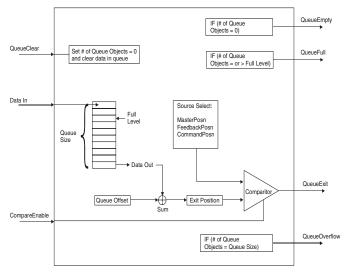
Figure 80: Queue Block Diagram
